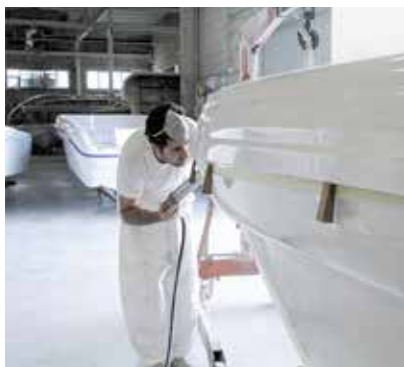
Fig. 102 Sealing with Sikaflex®-295 UV
