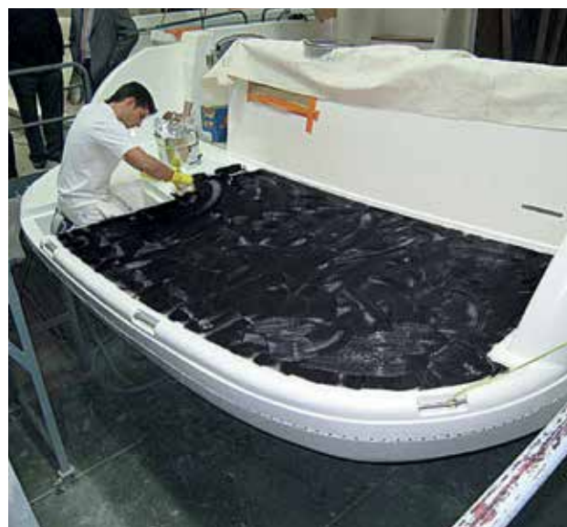
Fig. 52 Application of Sikaflex®-298
