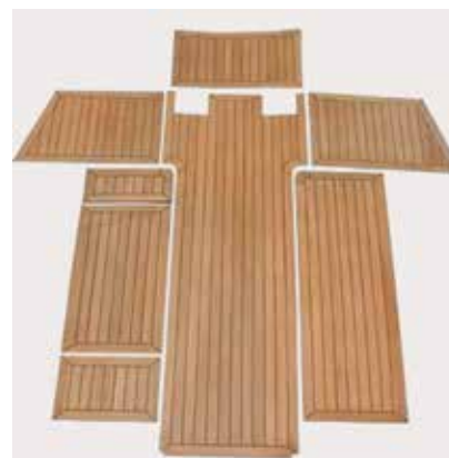
Fig. 48 A prefabricated teak deck is laid out in preparation for fitting
