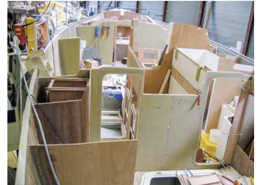
Fig. 93 Lightweight panels being fitted to an open hull
