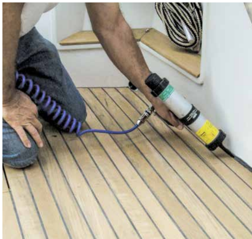
Fig. 51 Sealing the edges after renovation with Sikaflex®-295 UV
