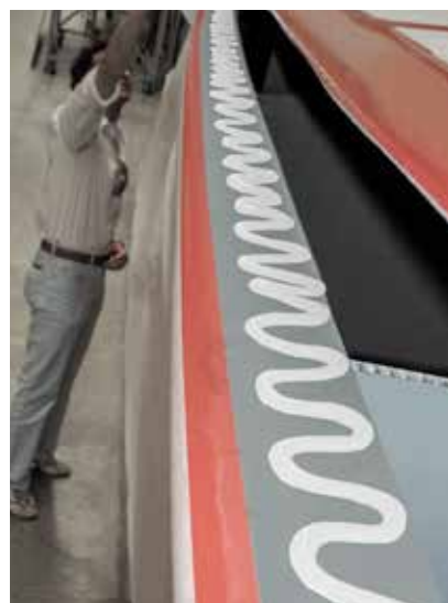
Fig. 103 Hull and deck are brought together
