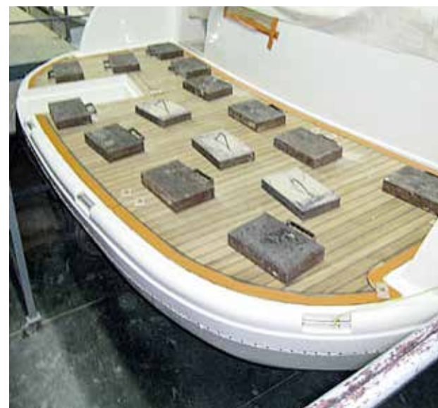
Fig. 53 Holding in place with weights
