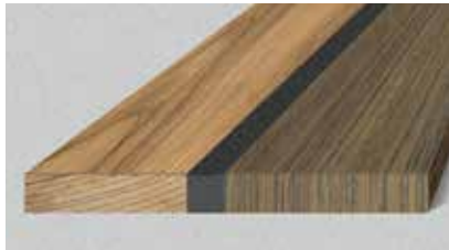
Fig. 27 Left side: laying year rings are not recommended. Right side: standing year rings are best.
