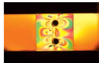
Fig. 5 Same sample plan view. Here stress concentration around the bolts is visible (stress peaks around the screw).
