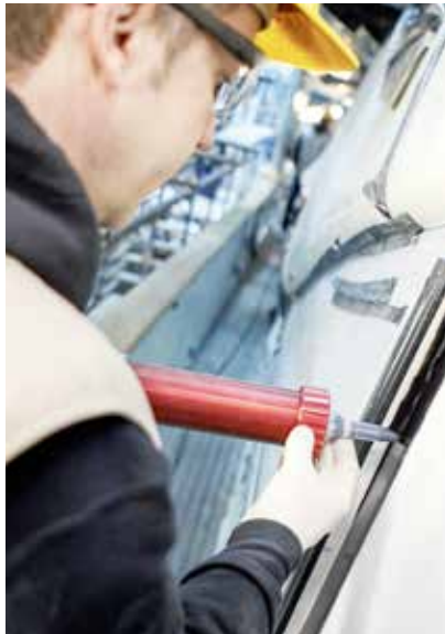
Fig. 100 Adhesive is applied to the window frame
