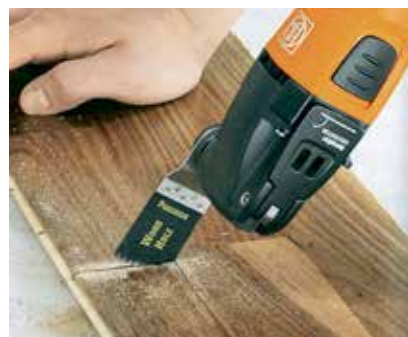
Fig. 74 Cutting planks with vibrating knife
