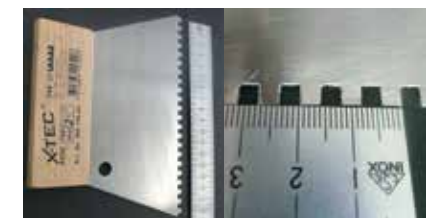
Fig. 37 Hand application picture comb trowel and comb trowel detail
